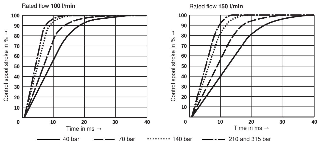
Frequency response with pressure rating 315 bar
